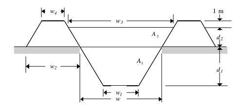
Design of the water channel presented in HW # 1 is to be performed using Sequential Linear Programming (SLP). The objective is to minimize the excavated area,  $A_1$ , which is equal to the material used for the dykes. It is also required that the wet-section cross sectional area is at least 150.0  $m^2$ . Also, the water depth in the canal,  $d_1 + d_2$ , must be larger than 15 m.
